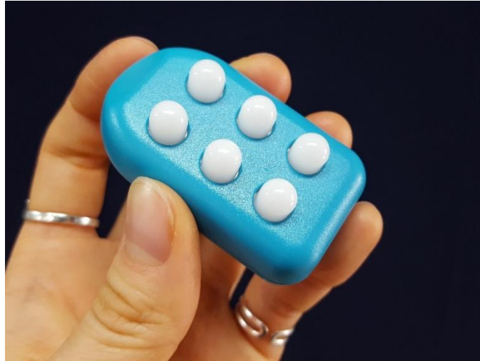
<Image: A left hand holding a taptile block with with all six dots pushed up>
